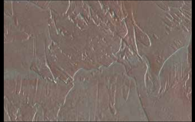
METEORE 8 (LT. 1) + COLORI' Col. 425 C (20 ML.) LAME' Col. 252 LAME' Col. 250 METEORE 8 (LT. 4) + COLORI' Col. 425 C (80 ML.) LAME' Col. 252 LAME' Col. 250
