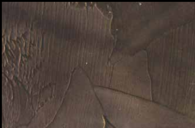
METEORE 8 (LT. 1) + COLORI' Col. 461 A (80 ML.) LAME' Col. 259 LAME' Col. 251 METEORE 8 (LT. 4) + COLORI' Col. 461 A (320 ML.) LAME' Col. 259 LAME' Col. 251
