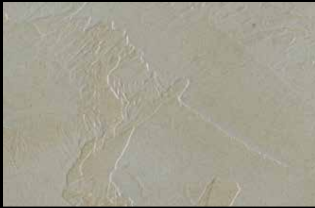
METEORE 8 (LT. 1) + COLORI' Col. 425 D (5 ML.) LAME' Col. 256 LAME' Col. 254 METEORE 8 (LT. 4) + COLORI' Col. 425 D (20 ML.) LAME' Col. 256 LAME' Col. 254
