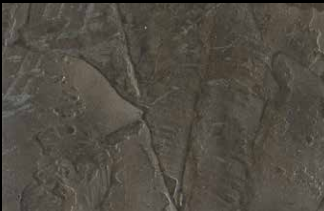
METEORE 8 (LT. 1) + COLORI' Col. 461 A (80 ML.) LAME' Col. 251 LAME' Col. 250 METEORE 8 (LT. 4) + COLORI' Col. 461 A (320 ML.) LAME' Col. 251 LAME' Col. 250
